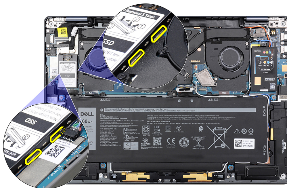
Figure 25. Solid state drive shielding cover
