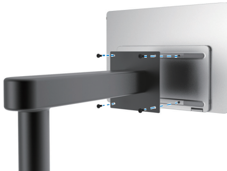
Figure 8. Attach the mounting bracket
