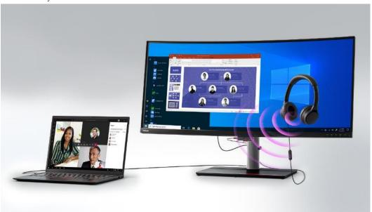
When plug off the earphone, the PC will not delivery the audio signal to monitor, it will delivery to other speakers connecting to PC. (internal or external speakers of PC)
